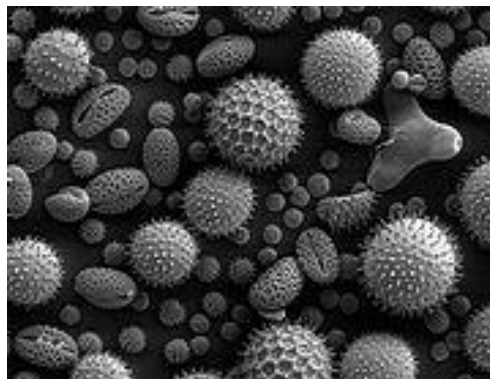
Fig.3: SEM picture of pollen grains show the characteristic depth of field of SEM micrographs
